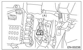
4) Connect the general scan tool to its data link connector.
