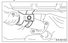
9) Remove the front and center exhaust pipe assembly from the vehicle.
