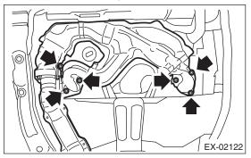
8) Remove the bolt which holds center exhaust pipe to hanger bracket.
