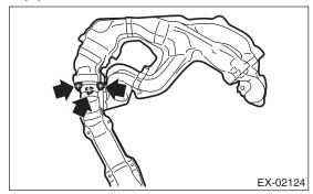
11) Remove the front oxygen (A/F) sensor and rear oxygen sensor. <Ref. to FU(H4SO)-36, REMOV-AL, Front Oxygen (A/F) Sensor.> <Ref. to FU(H4SO)-38, REMOVAL, Rear Oxygen Sensor.>
