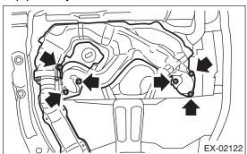
5) Tighten the bolt which holds the center exhaust pipe to exhaust pipe.
