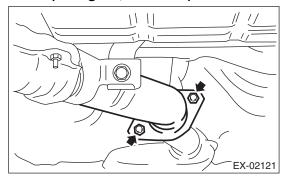
6) Tighten the bolt which holds center exhaust pipe to hanger bracket.
