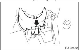
(5) Place the power steering pump on the right side wheel apron.
