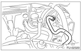
13) Connect the engine coolant hoses (A) to throttle body.
