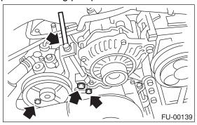
(3) Disconnect the connector (A) from power steering pump switch.
