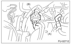
12) Disconnect the connectors from the engine coolant temperature sensor.
