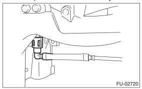
4) Install the fuel injector.
