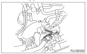
(3) Install the installation bolt of the power steering pump bracket.
