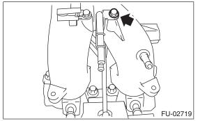
6) Install the engine harness onto intake manifold.
