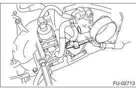
14) Disconnect the connector from crankshaft position sensor.
