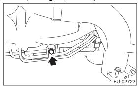
2) Connect the fuel injector pipe LH to the fuel pipe.
