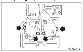
2) Connect the fuel hose and evaporation hose to the fuel pipe.
