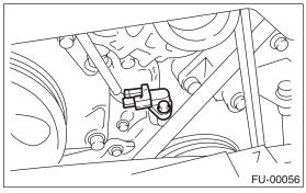
15) Disconnect the connector from the oil pressure switch (A).
