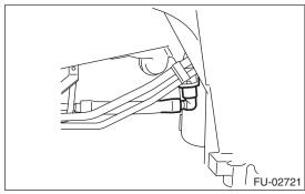
3) Connect the fuel injector pipe RH to the fuel pipe.
