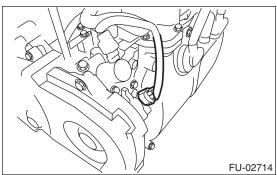
5) Connect the connector to the power steering pump switch.
