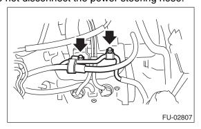
(2) Remove the installation bolt installing the power steering pump bracket.
