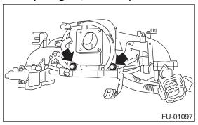
8) Hold the engine harness using the harness band clips.
