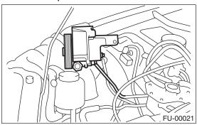
7) Remove the spark plug cords from the spark plugs by pulling the plug caps. (Do not pull the cord.)
