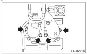
20) Remove the intake manifold.
