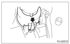
(2) Connect the power steering pump switch to the connector (A).
