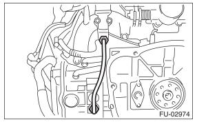
4) Connect the connectors to camshaft position sensor.
