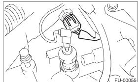
10) Connect the PCV hose (A) to intake manifold.
