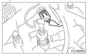
4) Remove the engine coolant temperature sensor.
