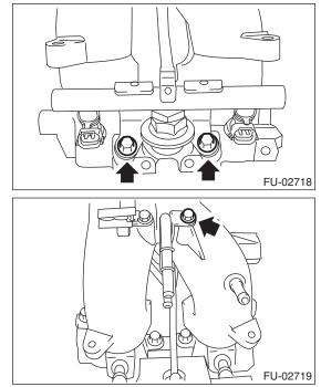
9) Remove the fuel injector while lifting up the fuel injector pipe.
