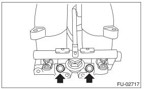
11) Remove the fuel injector while lifting up the fuel injector pipe.
