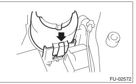
(6) Place the power steering pump and tank on the right side wheel apron.
