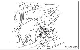
(5) Remove the power steering reservoir tank from the bracket by pulling it upward.
