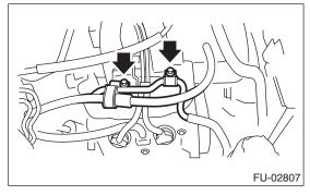
(3) Remove the bolts which install the power steering pump to the bracket.
