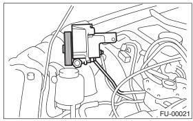
6) Remove the spark plug cords from spark plugs (#1 and #3 cylinders).
