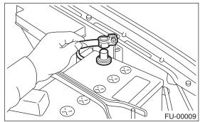
3) Remove the clip fastening the harness and disconnect the front oxygen (A/F) sensor connector.
