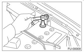
3) Remove the clip fastening the harness and disconnect the rear oxygen sensor connector.
