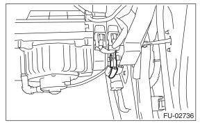
5) Remove the main relay from the mounting bracket.
