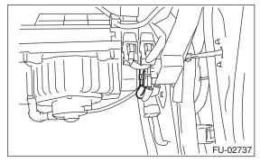
5) Remove the fuel pump relay from the mounting bracket.
