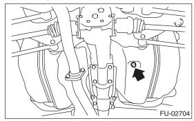
6) Tighten the fuel drain plugs.
