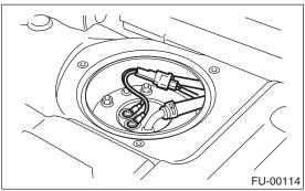
9) Remove the bolts which install fuel sub level sensor on fuel tank.
