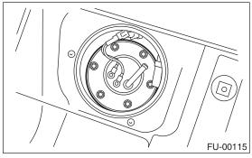
10) Remove the fuel sub level sensor.
