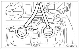
4) Remove the spark plug with a spark plug socket.
