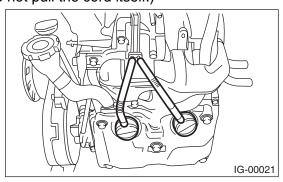
3) Remove the spark plug with a spark plug socket.
