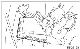
Fasten with a clip after inserting the lower tab of case.
