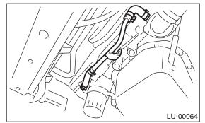
7) Remove the radiator. <Ref. to CO(H4SO)-27, REMOVAL, Radiator.>
