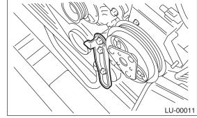
11) Remove the crank pulley using ST. ST 499977100 CRANK PULLEY WRENCH
