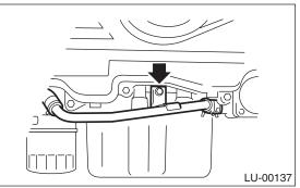
6) Remove the water pipe and hoses between oil cooler and water pump. (Turbo model)
