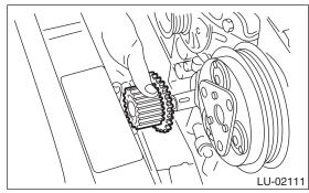
15) Remove the bolts which install oil pump onto cylinder block.
