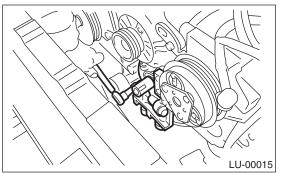
16) Remove the oil pump by using flat tip screwdriver.
