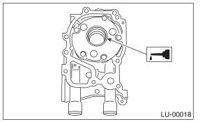
4) Position the oil pump, aligning the notched area with crankshaft, and push the oil pump straight.
