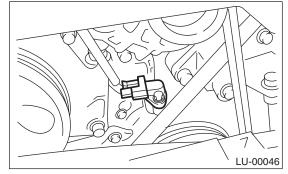
9) Remove the V-belts. (Non-turbo model) <Ref. to ME(H4SO)-40, REMOVAL, V-belt.> (Turbo model) <Ref. to ME(H4DOTC)-40, REMOVAL, V-belt.> 10) Remove the V-belt tensioner.
