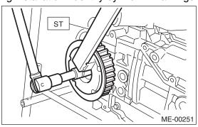
2) Install the cam sprocket No. 2. To lock the camshaft, use the ST.
