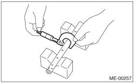
2) If the oil clearance exceeds the limit, replace the valve rocker arm or shaft, whichever shows greater amount of wear.
