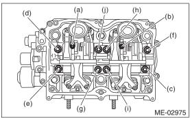
(3) Remove the valve rocker assembly.
