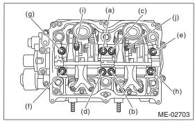
(4) Use the ST to rotate the spring stopper in the direction of the arrow to fasten the adjuster pin.
