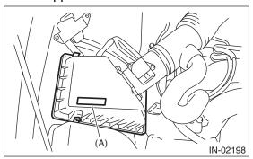
•Fasten with a clip after inserting the lower tab of case.
