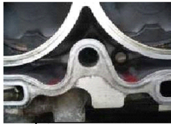
After cleaning coolant sealing portion (block)
