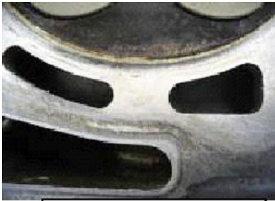
After cleaning oil sealing portion (head)
