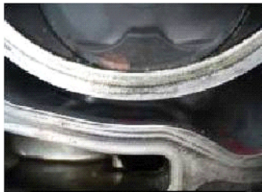
After cleaning oil sealing portion (block)
