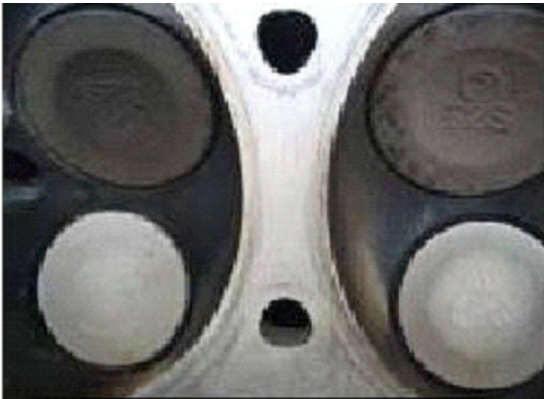
After cleaning bore sealing portion (head)
