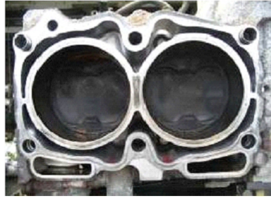
Finished cleaning (block)
