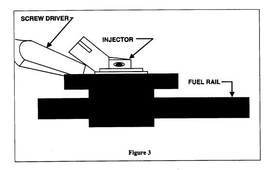
6. Remove the fuel injector(s) and place it in the box that contained the new injector(s) or wrap it to protect it during return shipping and handling. Any injectors received damaged will not be accepted.
