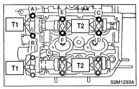
(4) Similarly, tighten the cap on exhaust side. After tightening the cap, ensure the camshaft rotates only slightly while holding it at "base" circle.
