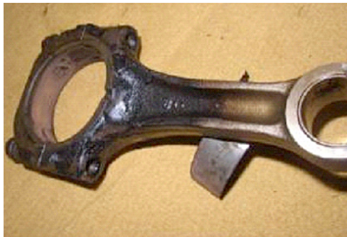
Rod Bearing Spun from Lack of Oil
