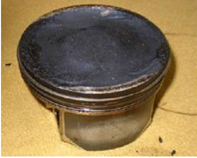
Ring Land Damage from Detonation
