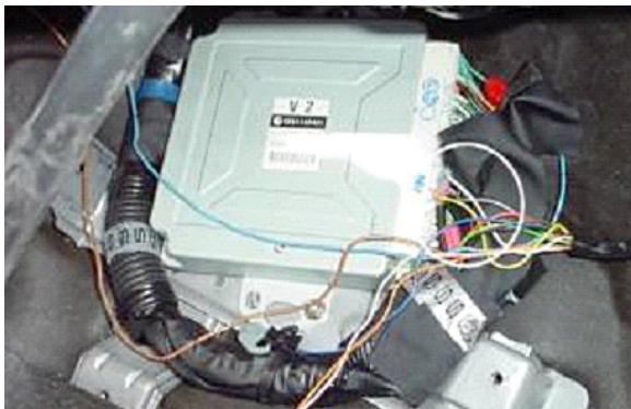
Aftermarket Air Fuel Controller wired to ECM
