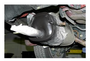
7. Remove tape and paper, reinstall muffler to rubber mounting.
