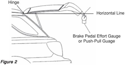
This chart provides specifications to determine if the rear gate stay(s) has failed.
