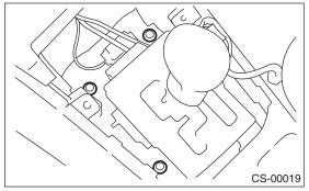
3) Install the console box. <Ref. to EI-36, INSTAL-LATION, Glove Box.>
