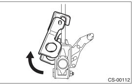
17) Remove the bushing from the bracket.
