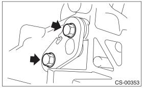
9) Remove the lock plates A, B, and C and the bushing.
