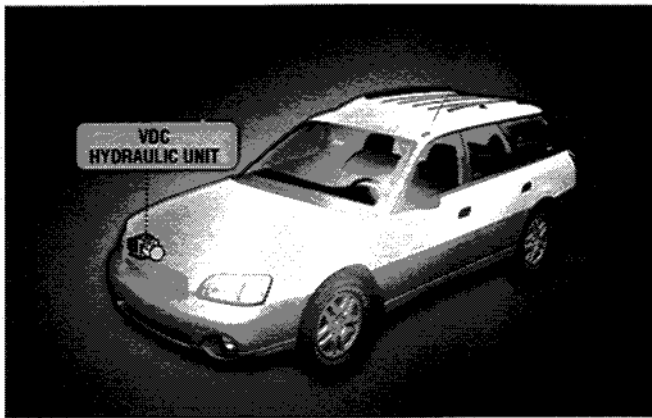
Location of VDC Hydraulic Unit
