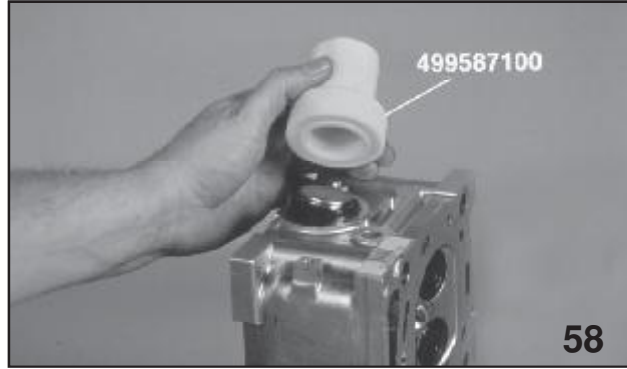
Installing the Oil Seal
