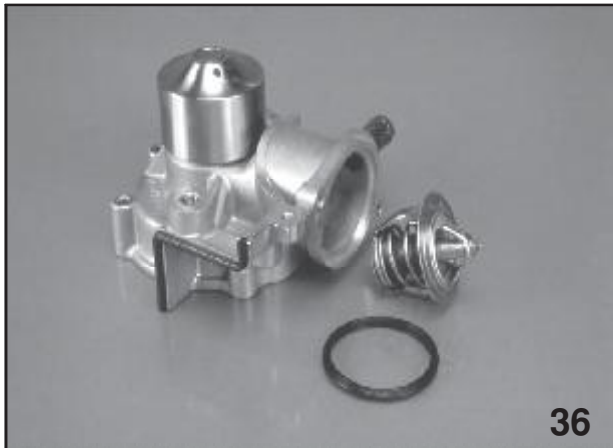
Water Pump Assembly-Cooling System
