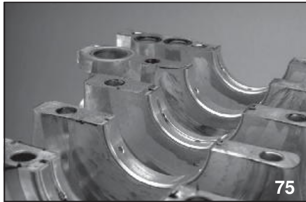
Main Bearing Oil Grooves
