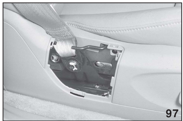
Seat belt Anchor Cover Removed
