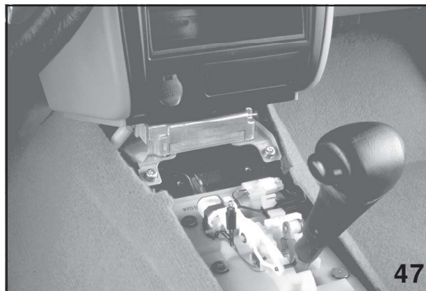
Control Unit Location
