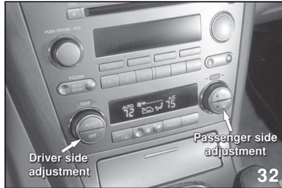
HVAC Display Panel
