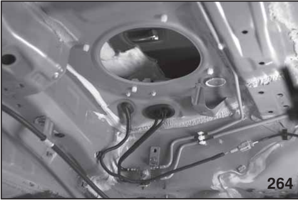
Tank Removed, Main Pump Access
