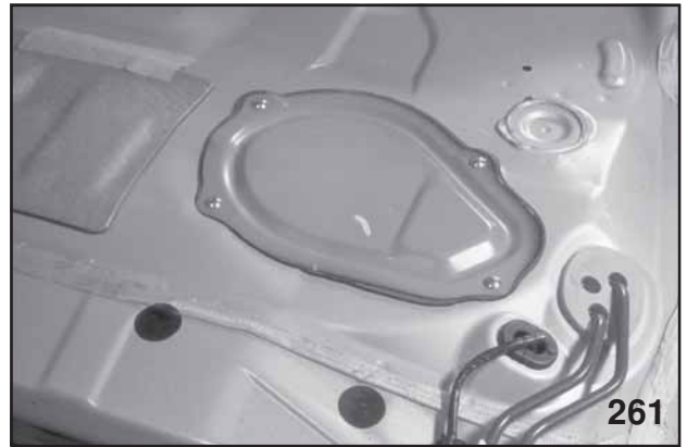
Sub Pump Access
