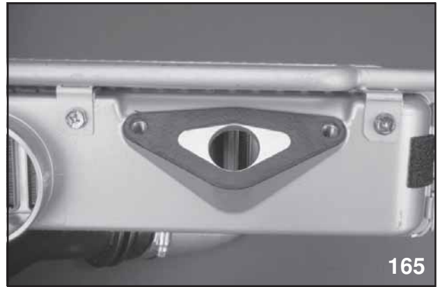
Bypass Valve Connection
