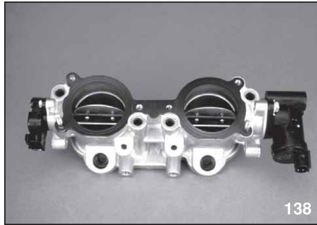
Tumble Generator Valve Rail
