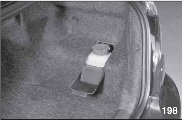
Normal Access to the Water Tank
