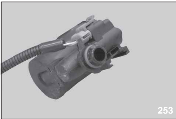
Drain Valve Separated from Canister (NOT SERVICEABLE)
