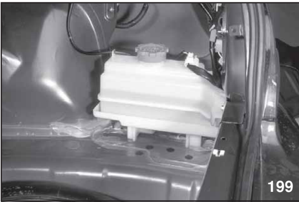
Water Tank Complete
