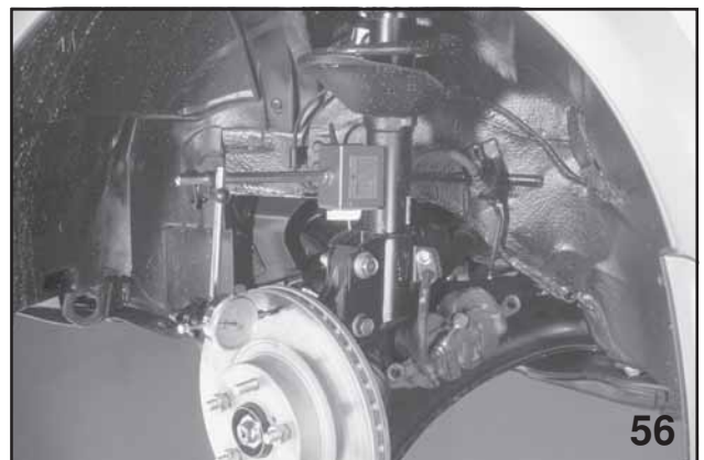
Measuring Rotor Runout
