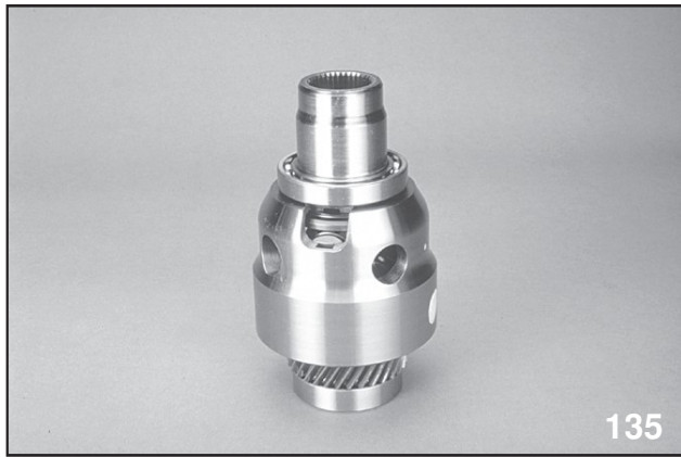
1999 and Later Center Differential Assembly
