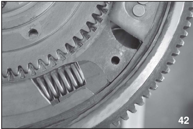
Actuator in contact with Spring Carrier
