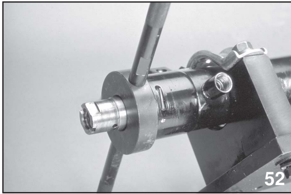
Locate end of Circlip
