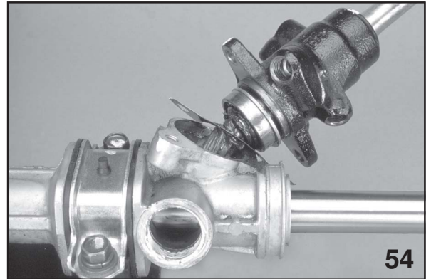
Removing Control Valve
