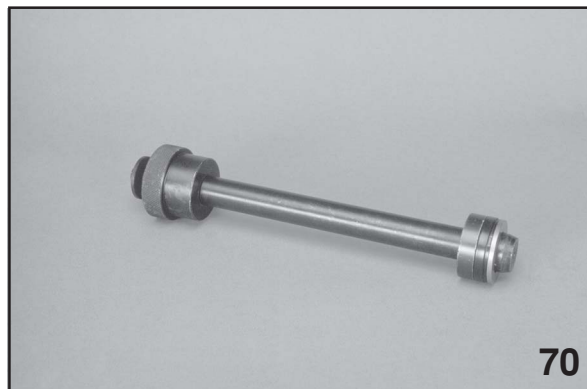
Inner Seal and Backing Washer on tool
