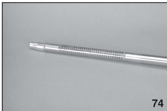
Rack Cover installed
