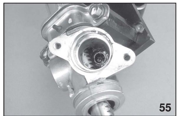
Control Valve Removed
