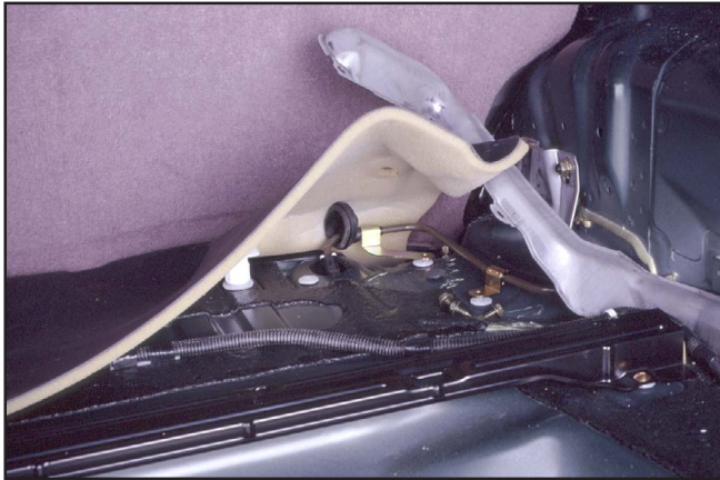
Quick Connector on Vent Hose (Located in cargo area of station wagon, trunk of sedan.)
