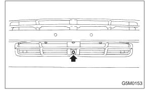
7) Remove bolt from lower center of bumper.
