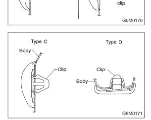
Type C: Protector is attached to body with clips.
