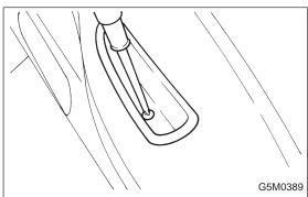
4) Remove pull handle attaching screw and then remove pull handle.
