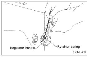
2) Remove retainer spring and then regulator handle. Use a wire bent at one end, as shown in figure, for easier removal of retainer spring. (models without power window)
