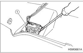
9) Disconnect data link connector 1) from lower cover.
