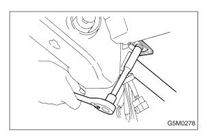
13) Remove two bolts and lower steering column.
