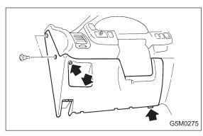
8) Remove lower cover and then disconnect seat belt timer connector.
