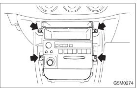
7) Remove audio assembly and then disconnect radio antenna feeder and connectors.
