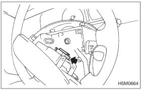
5) Disconnect airbag and horn connectors on back of airbag module. <Ref. to 5-5 [M2-6].>
