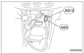
4) Disconnect airbag connector (AB9) and (AB10) <Ref. to 5-5 [T5F1].>
