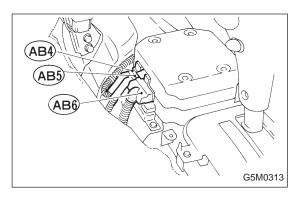
5) Remove instrument panel console. <Ref. to 5-4 [W1A0].> Disconnect 12-pin yellow connector (AB6) from airbag control unit. <Ref. to 5-5 [M2-6].>
