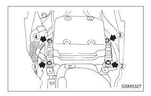
6) Using TORX  $\!^{\tiny{\circledR}}$  BIT T30, remove four TORX  $\!^{\tiny{\thickspace}}$  bolts in numerical sequence shown in figure.
