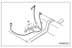
7) Roll up floor mat and side sill cover. (LH side). Remove main harness from clip and protector.
