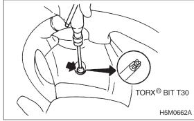
5) Set front wheels in straight ahead position. Using TORX® BIT T30, remove two TORX® bolts.
