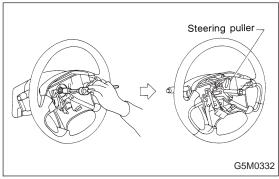
7) Using steering puller, remove steering wheel.
