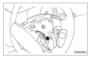
6) Disconnect airbag connector and horn connector on back of airbag module. Remove airbag module, and place it with pad side facing upward. <Ref. to 5-5 [W102].>
