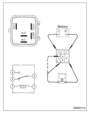
Check continuity between terminals (indicated in table below) when terminal (1) is connected to battery and terminal (2) is grounded.
