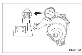
2) Check wiper motor operation at high speed. Connect battery wiper motor. Check wiper motor for proper operation at high speed.
