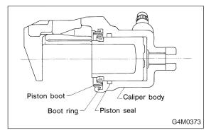
6) Install the piston boot to the caliper body, and attach boot ring.
