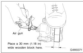
3) Gradually supply compressed air via inlet of caliper body to force piston out.
