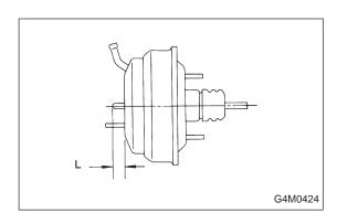
(2) Whether or not reaction disc has dropped can be determined by measuring the dimension "L".
