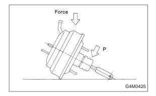
4) Use care when placing brake booster on the floor.
