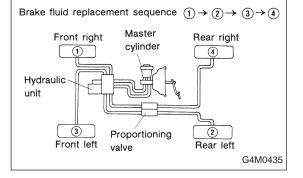
5) Install one end of a vinyl tube onto the air bleeder of and insert the other end of the tube into a container to collect the brake fluid.
