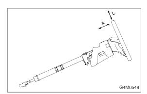
2) Check steering wheel free play in axial and radial directions:
