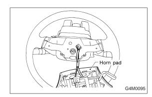
9) Install horn pad to steering wheel. (without airbag model)
