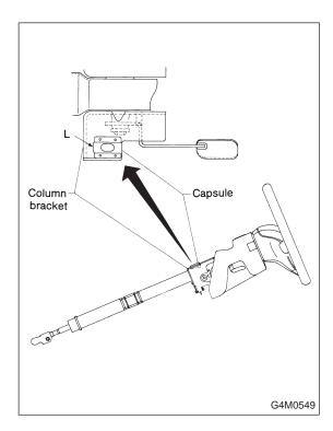
5) Check to ensure that clearance between capsule (at steering column) and cutout portion of column bracket on steering column upper side is within specifications.
