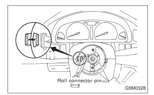
6) Align center of roll connector. (with airbag model) <Ref. to 5-5 [W501].>
