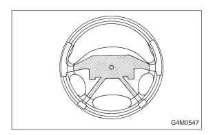
1) Check steering wheel insert for cracks or deformities.
