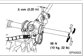
Left-turn steering: Service limit Direction ◊ ◊ 0.3 mm (0.012 in) or less Direction ← → 0.15 mm (0.0059 in) or less
