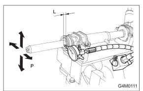
2. RACK SHAFT PLAY IN RADIAL DIRECTION Right-turn steering:
