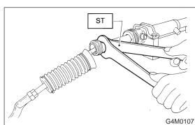
6) Fit new lock washer on screwed portion of rack end. Aligning cut portion of rack and nail of washer, screw in and tighten ball joint by using ST and spanner.
