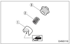
5) Apply grease to sliding surface of sleeve and spring seat, then insert sleeve into pinion housing. Fit spring into sleeve screw, pack grease inside of screw, then install the screw.
