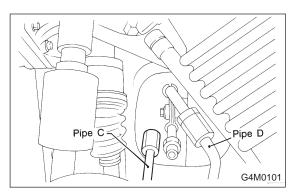
9) Disconnect pipes C and D from pipe of gearbox.
