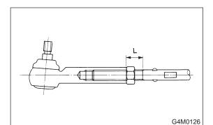
14) If tie-rod end was removed, screw in lock nut and tierod end to screwed portion of tie-rod, and tighten lock nut temporarily in a position as shown in figure.
