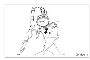
In axial direction: Service limit 0.1 mm (0.004 in) or less On condition P: 20 — 49 N (2 — 5 kg, 4 — 11 lb)
