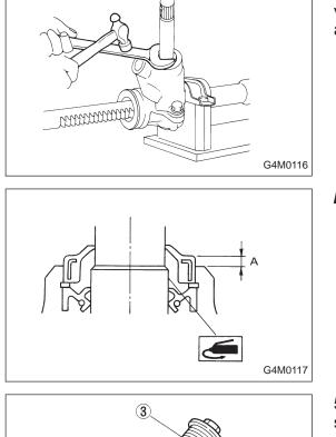
4) Press-fit dust seal into gearbox housing while tapping it via a spanner or the like so that stepping between gearbox and dust seal is normally 2 mm (0.08 in).
