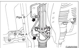
7) Remove one pipe joint at the center of gearbox, and connect vinyl hose to pipe and joint. Discharge fluid by turning steering wheel fully clockwise and counterclockwise. Discharge fluid similarly from the other pipe.
