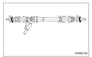
4) If steering wheel spokes are not horizontal with vehicle set in the straight ahead position after this adjustment, correct it by turning the right and left tie-rods in the same direction by the same turns.
