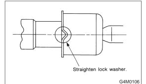
6) Straighten lock washer under ball joint.
