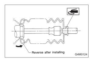
12) Turn boot until it seats well on gearbox and rubber mounting, then bend boot flange back.
