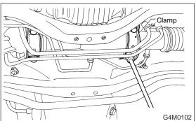
10) Remove clamp bolts securing gearbox to crossmember, and remove gearbox.
