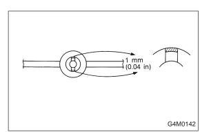
Rack ASSY Rack stopper G4M0143 NOTE: If ST is used, grind area (shown in figure) by 1 mm (0.04 in) in advance.
