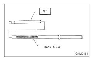
2) Fit ST over toothed portion of rack assembly, and check for binding or unsmooth insertion. If any deformation is noted on flats at the end of rack, shape by using file, and wash with cleaning fluid.
