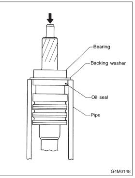
2) Press out bearing together with backing washer using pipe of I.D. 38.5 to 39.5 mm (1.516 to 1.555 in) and press. **CAUTION:**
