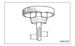
(1) Check at temperature  $21^{\circ}C$  (70°F) on reservoir surface of oil pump, read the fluid level on the "COLD" side.
