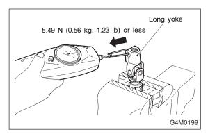
NOTE: Measurement of folding torque of universal joint
