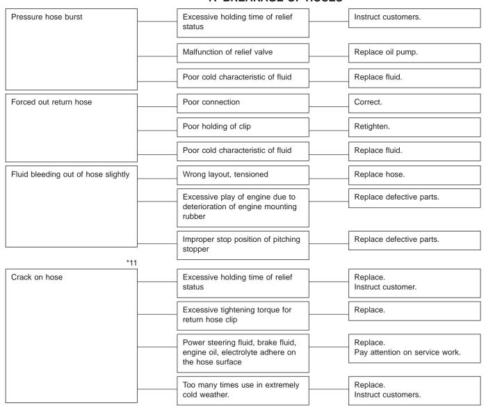
\*11 Although surface layer materials of rubber hoses have excellent weathering resistance, heat resistance and resistance for low temperature brittleness, they are likely to be damaged chemically by brake fluid, battery electrolyte, engine oil and automatic transmission fluid and their service lives are to be very shortened. It is very important to keep the hoses free from before-mentioned fluids and to wipe out immediately when the hoses are adhered with the fluids.
